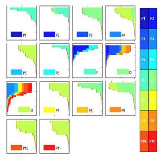
Well controls for the optimized production strategies presented in above figure. Well names refer to the positions in the initial configuration. Notice that there are more than one optimal well position in this problem because of symmetry and because the Lorenz coefficient is not convex.
