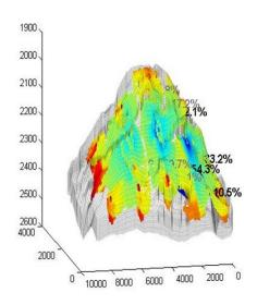
The figures presents Chemical flood optimization for a shallow marine reservoir. Initial time steps, indicating that the major changes in the reservoir happen when the initial front starts to propagate.
